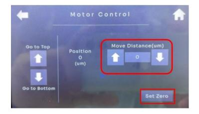
Example 1: - Note down the gap values of the four corners measured by the printing platform (Picker/Build Platform) as shown in Table 1. Enter 200 in the motor control and press set zero Afterwards, move the printing platform (Picker/ Build Platform) up and down completely once, then measure the Gap as shown in Table 2, which meets the specifications.
